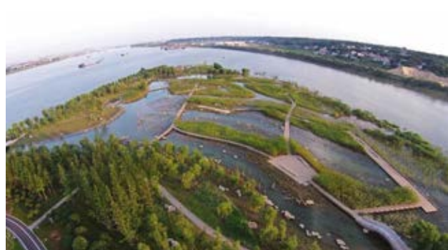
Variable grading makes the flood fluctuation no longer a threat, offering instead an opportunity for increasing biodiversity. Different water levels contribute to various habitats. This image shows the south wetland in summer with high water level.
