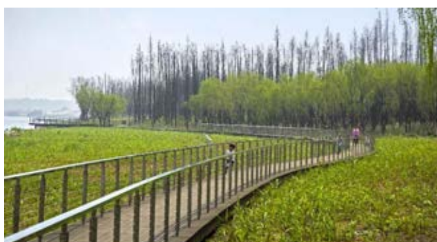
Trails and boardwalks lead the visitors through a meandering journey of discovery. Hidden surprises await in the forest, while commanding views define the wetland experience. Local condensed bamboo, a light-weight material resistant to flooding, is employed.
